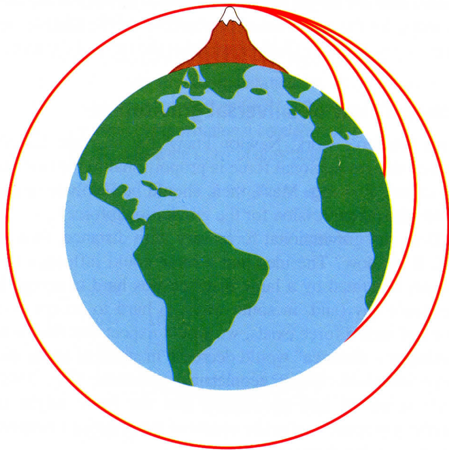
figure 5.17 In a diagram similar to this, Newton imagined a projectile fired from an incredibly high mountain. If fired with a large enough horizontal velocity, the projectile falls toward the Earth but never gets there.
